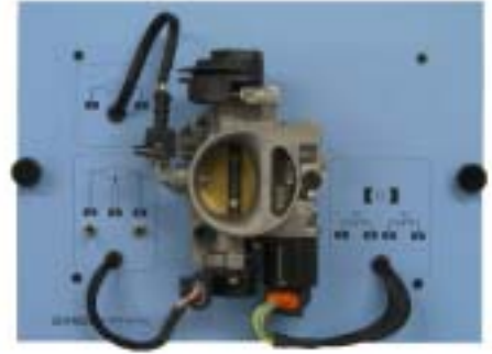
Magneti Marelli butterfly housing with stepper motor, air CTN and butterfly recopy potentiometer.
