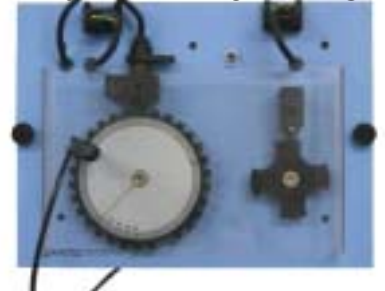
Toothed wheel with inductive Sensor and Hall effect sensor.
