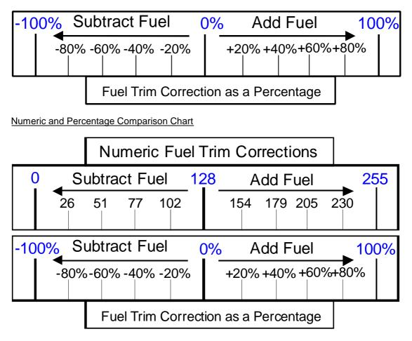
OBD II has specific monitoring of the fuel trim corrections. If the system detects problems with the air/fuel ratio, the system will log a Data Trouble Code (DTC) and turn on the vehicle dashboard Malfunction Indicator Lamp (MIL).
