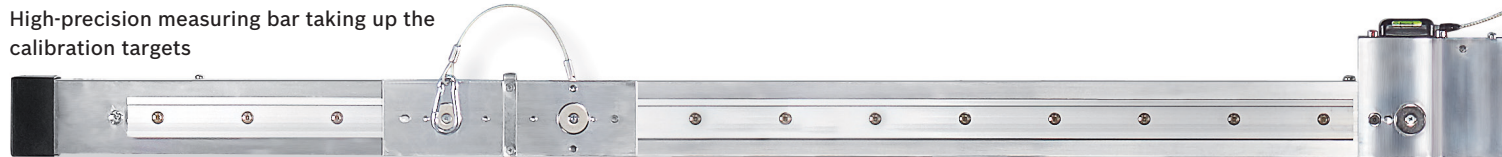
VAS 6430 adjustment device with fitted DAS modules and 3D measurement boards
