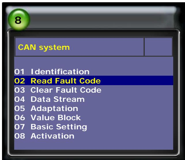
5. Confirm **No Fault Code** in Parking Brake system, then select **Basic Setting**
